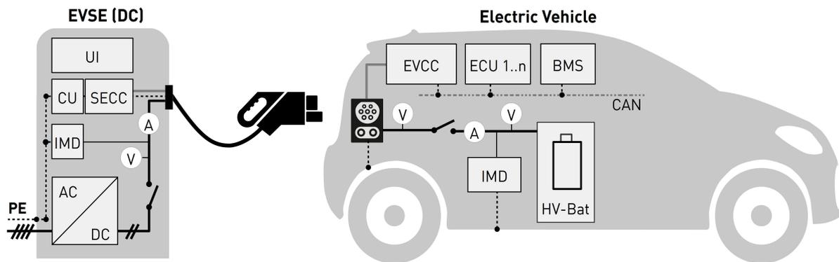
**Figure 2: Charging System of EVSE and EV**
