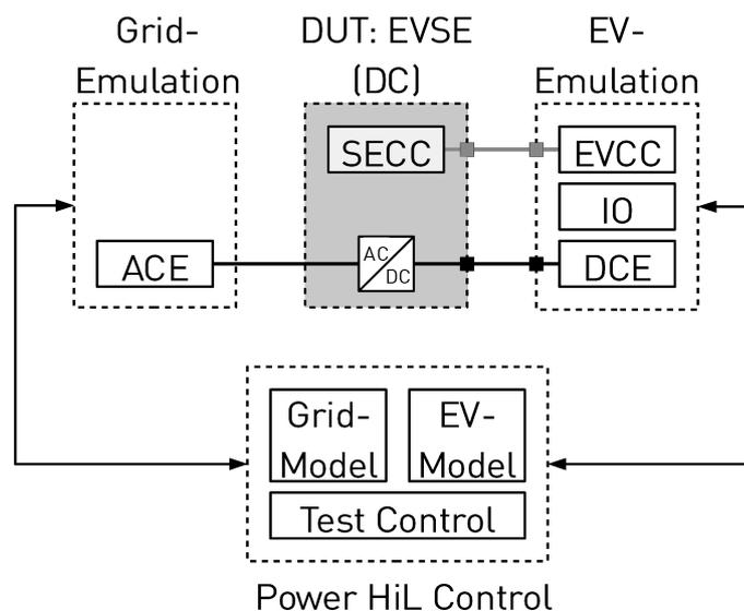
**Figure 3: Power HiL Test Environment (for DC EVSE)**
